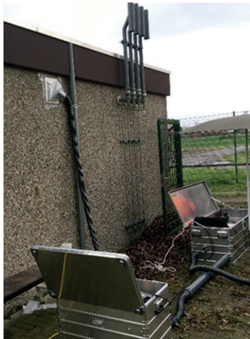
Figure 3 (left): Measurement Using the Suction Method at a Gas Pressure Regulating and Metering Station
