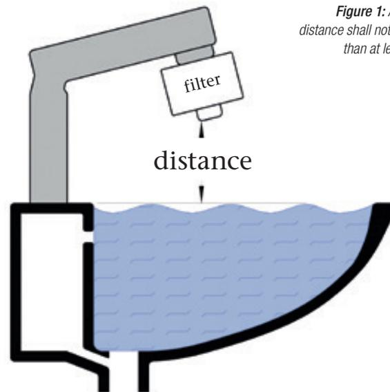
**Figure 1:** Air gap: the distance shall not be smaller than at least 20 mm
